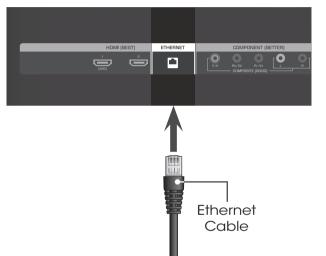
If you have a high-speed internet connection, connect an Ethernet cable from your modem or router to the back of the TV as shown.
